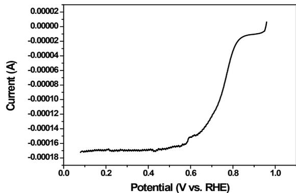
Multi-channel double electrode cell (m-CFDE)  $E_{1/2}$  agrees with RDE to 30 mV for PGM-free catalyst and within 9 mV for PGM catalyst. Automated deposition will improve agreement.
