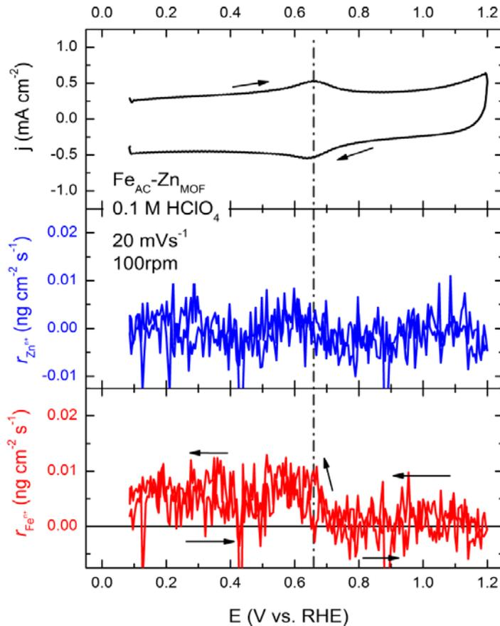
LANL (AD)Fe-N-C: 0.3 mg/cm<sup>2</sup>; potential cycling range: 0.08 - 1.2 V vs. RHE; RDE at 100 rpm
