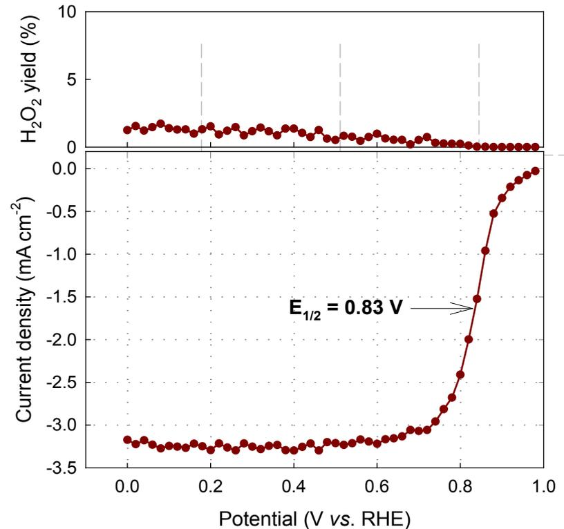
**Highlight:** Atomically dispersed Fe catalyst showing very high ORR activity in RDE testing ( $E_{1/2}$  of **0.83 V**) and excellent 4e<sup>-</sup> selectivity (H<sub>2</sub>O<sub>2</sub> yield < **1.5 %**)
