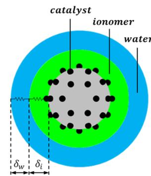
$O_2$  mass transport losses are dominated by flooded pores in thick electrodes and film resistance in thin electrodes
