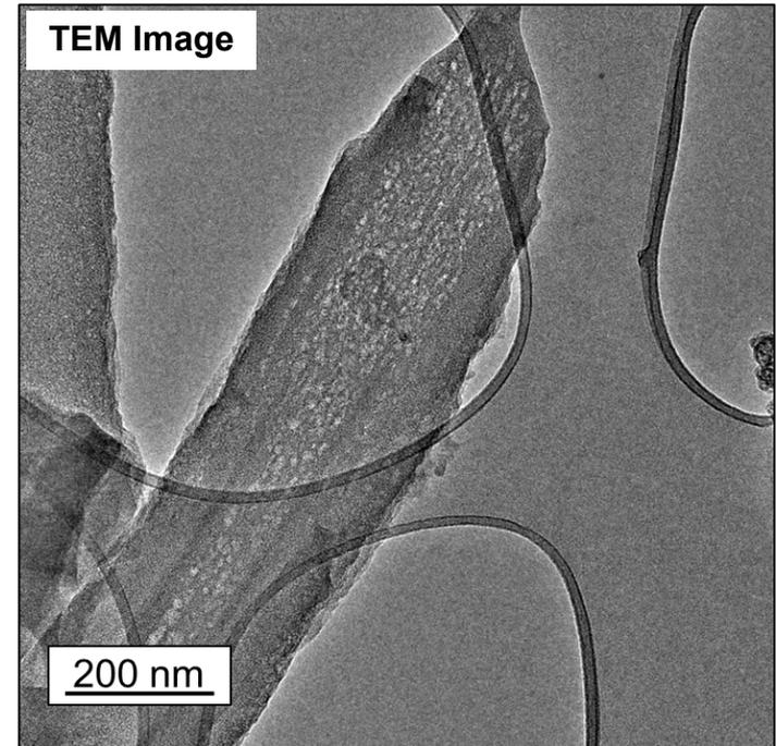
Carbon plates,  $\sim 0.2 \mu\text{m}$  wide and  $1.5\text{-}2.0 \mu\text{m}$  long, with enhanced microporosity due to Zn evaporation  $\rightarrow$  much improved accessibility to ORR active sites
