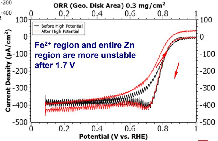
LANL (AD)Fe-N-C: 2.5 at% Fe, 1100°C, H<sub>2</sub>SO<sub>4</sub>-treated
