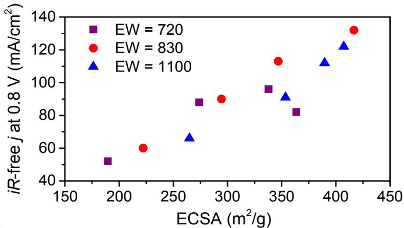
Increasing ionomer content from 25 wt% to 55 wt% improves kinetic performance thanks to higher catalyst utilization, *i.e.*, higher electrochemically-active surface area (ECSA)
