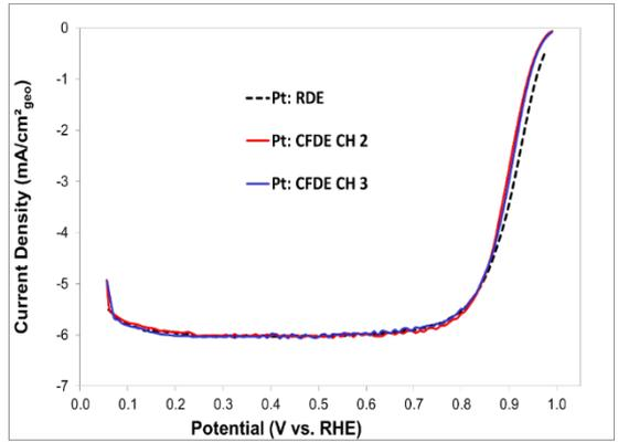
ORR, 18 μg<sub>Pt</sub>/cm<sup>2</sup> TKK 46 wt% Pt/C catalyst, 0.1 M HClO<sub>4</sub>
