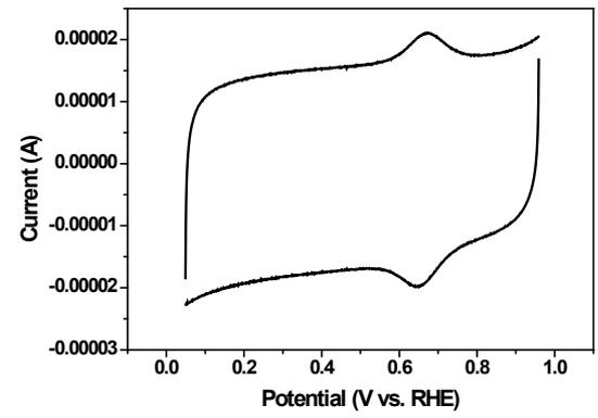
0.6 mg/cm<sup>2</sup> of LANL's (CM+PANI)-Fe-C(Zn) catalyst; 0.5 M H<sub>2</sub>SO<sub>4</sub>
