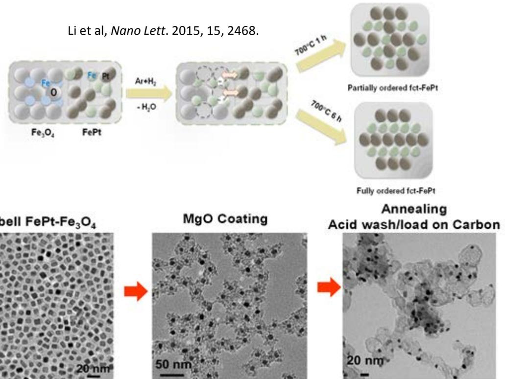
**MgO protection enables annealing to fully-ordered fct structure without particle growth**
