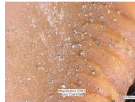
Failed valve seal
