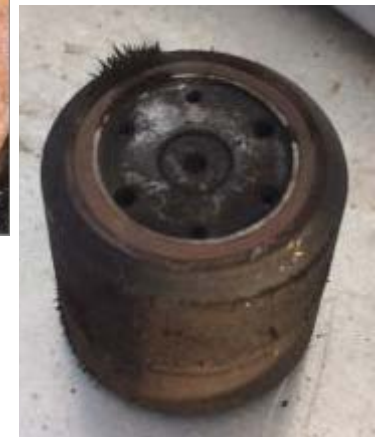
Failed check valve
