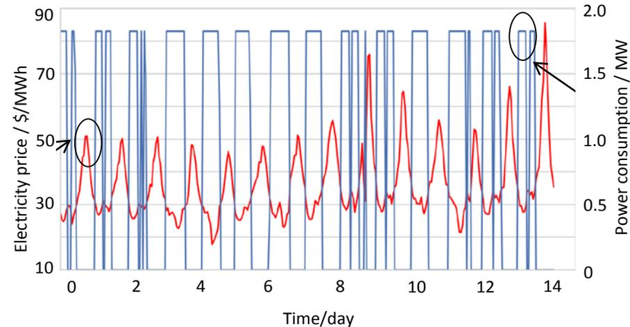
Example of cost-optimized operation of hydrogen electrolyzer that accounts for the dynamic price of electricity (using time-of-use electricity prices)
