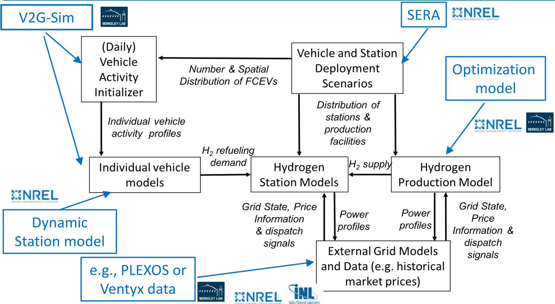
The H2VGI model integrates multiple operational and deployment models for FCEVs and H2 generation resources with external grid models across various time scales
