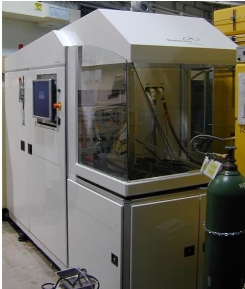
Large scale test stand: 800 W, 6-1000 A @ 0.2 V, 0 V – 50 V, Liquid coolant H<sub>2</sub>/Air: 11/27 slpm Contact humidifier (dew pt. 35-85 °C) First User Data 03/15
