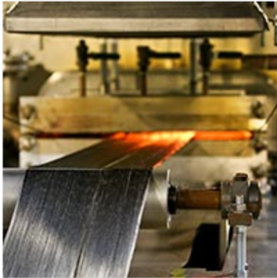
Oxidized fibers are converted into carbon fiber
