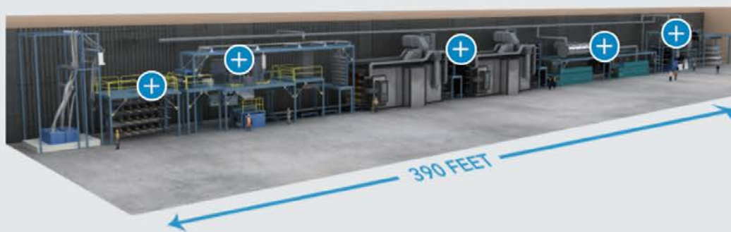
Oxidized fibers are converted into carbon fiber
