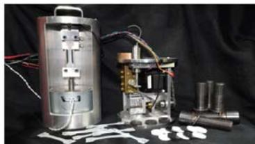
Tribology: A custom built linear reciprocating (ASTM G133) pin on flat system that is capable of testing samples up to approximately 1" wide at XN, and 5Hz with a stroke length of 1/8". The system was designed primarily for polymeric materials, but could potentially accommodate metals testing.
