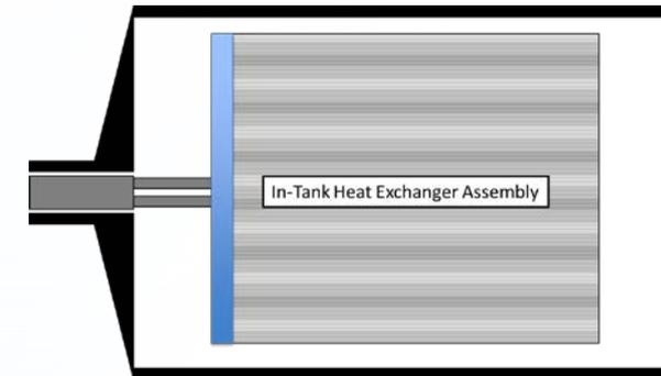
2. Insert pre-assembled heat exchanger and coolant port through the boss throat
