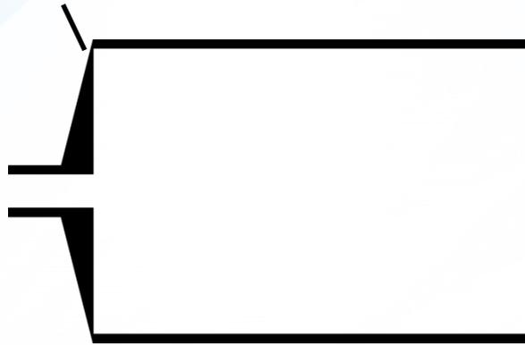
1. Assemble coolant-side dome and cylindrical section of tank liner
