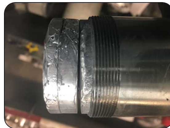
Aluminum foil coated 50 mm alane pellets after full hydrogen desorption from demonstration vessel
