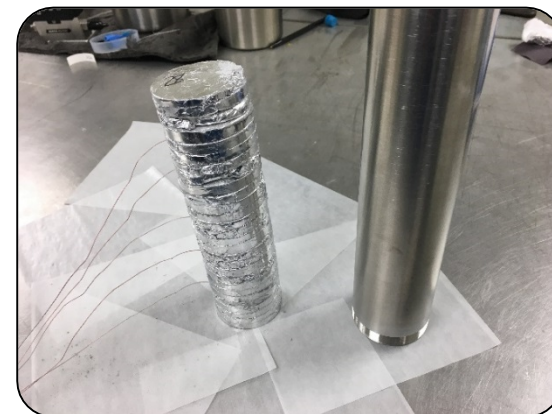
Aluminum foil coated 50 mm alane pellet stack with thermocouples
