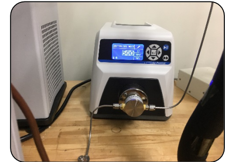
Gear pump used to simulate heat transfer fluid flow rates
