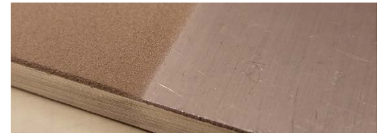
Aluminum 6061 substrate coated with commercially pure nickel using PNNL cold spray equipment
