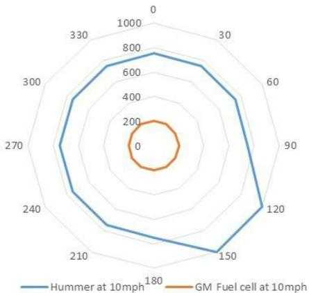
***By comparing two like vehicle systems (Colorado ZH2 & HMMWV) the fuel cell vehicle has a 75-90% improvement for its acoustic signature.***
