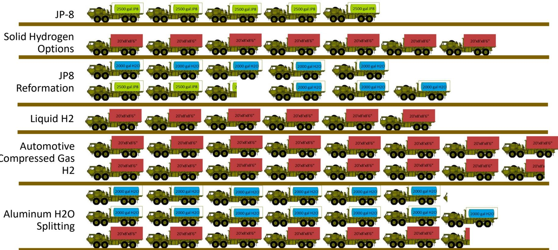
M1120 LHS Capacities, no trailers. Corrected for improved fuel consumer efficiency and H<sub>2</sub> to JP-8 energy difference. Compression of H<sub>2</sub> and fuel consumed by M1120 ignored.
