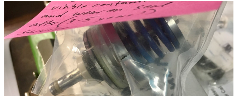
Field-failed 700 bar inlet valve
