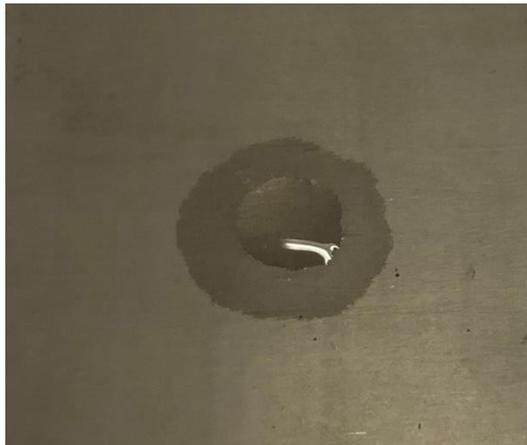
Water droplet on super-hydrophobic  $\text{TiO}_x$  coated SS plate.
