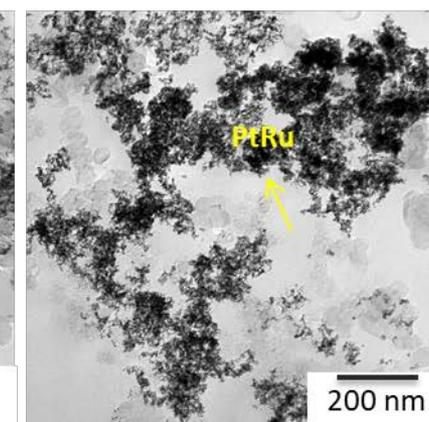
Unlike cathode, electrode structure remains similarly over the testing period at anode
