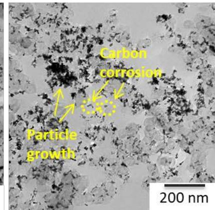
At cathode, obvious structural changes can be seen, e.g. pt particle growth and carbon corrosion over the testing period
