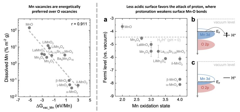
Acid stability descriptor developed for manganese oxides, indicating high stability of high oxidation state manganese oxides.
