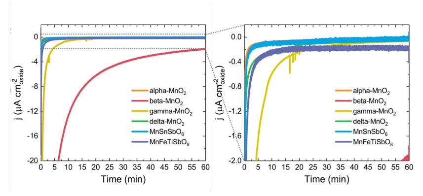
Activity of  $\beta$ -MnO<sub>2</sub> is significant over a 1-hour hold at 0.9 V (~2  $\mu$ A-cm<sup>-2</sup> vs. initial target 0.5  $\mu$ A-cm<sup>-2</sup>, final target 4.4  $\mu$ A-cm<sup>-2</sup>)
