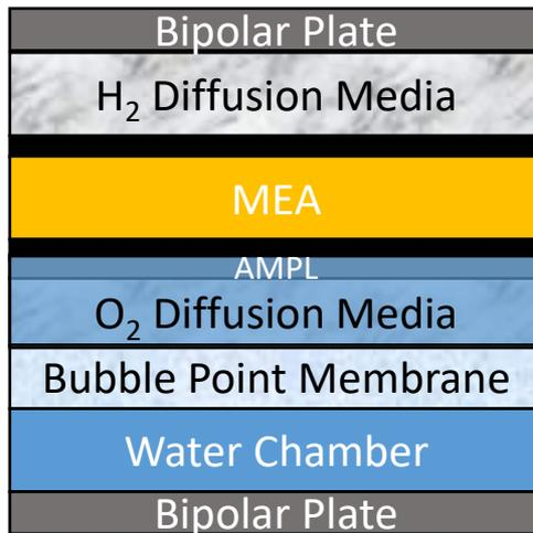
Oxygen chamber completely filled with high pressure circulating water in electrolyzer mode
