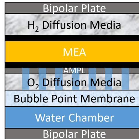
Water is removed from oxygen chamber via amphiphilic diffusion media and bubble point membrane in fuel cell mode under pressure gradient
