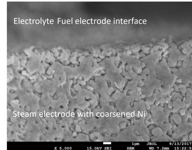
Delamination and Ni phase coarsening were evident from the cell tested under high steam conditions
