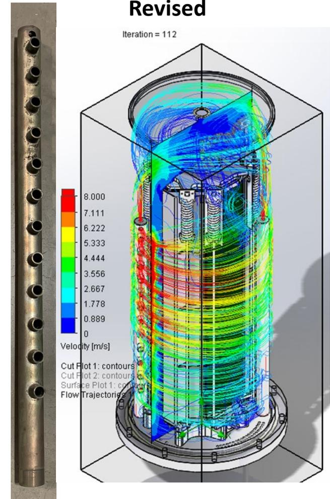
Test results suggested an air flow sensitivity. A re-examination of the air inlet distribution tubes showed a potential cause. Flow momentum at the higher flow rates was favoring air flow to the top. A revised air inlet was designed and built
