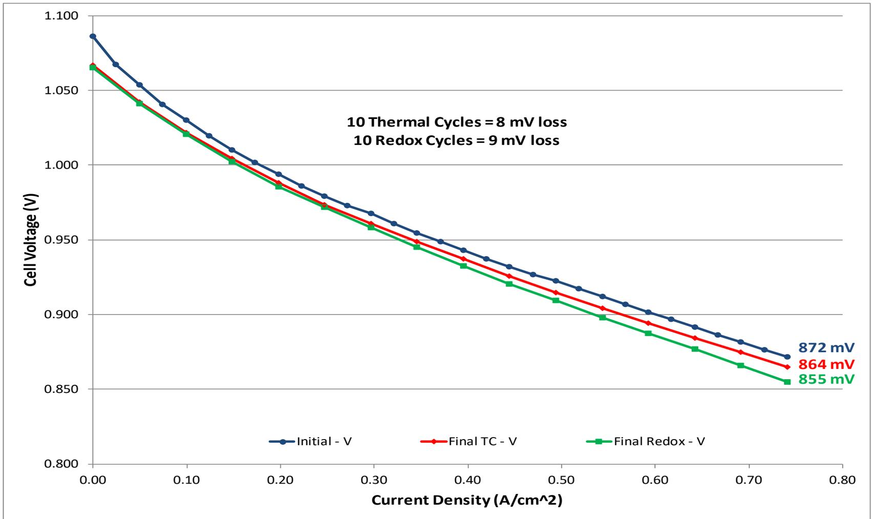
**Performance Curves Comparison at 750°C after 10 Thermal and 10 Redox Shutdown Cycles With 5 Hour Hot Holds (Fuel Pipes Disconnected)**
