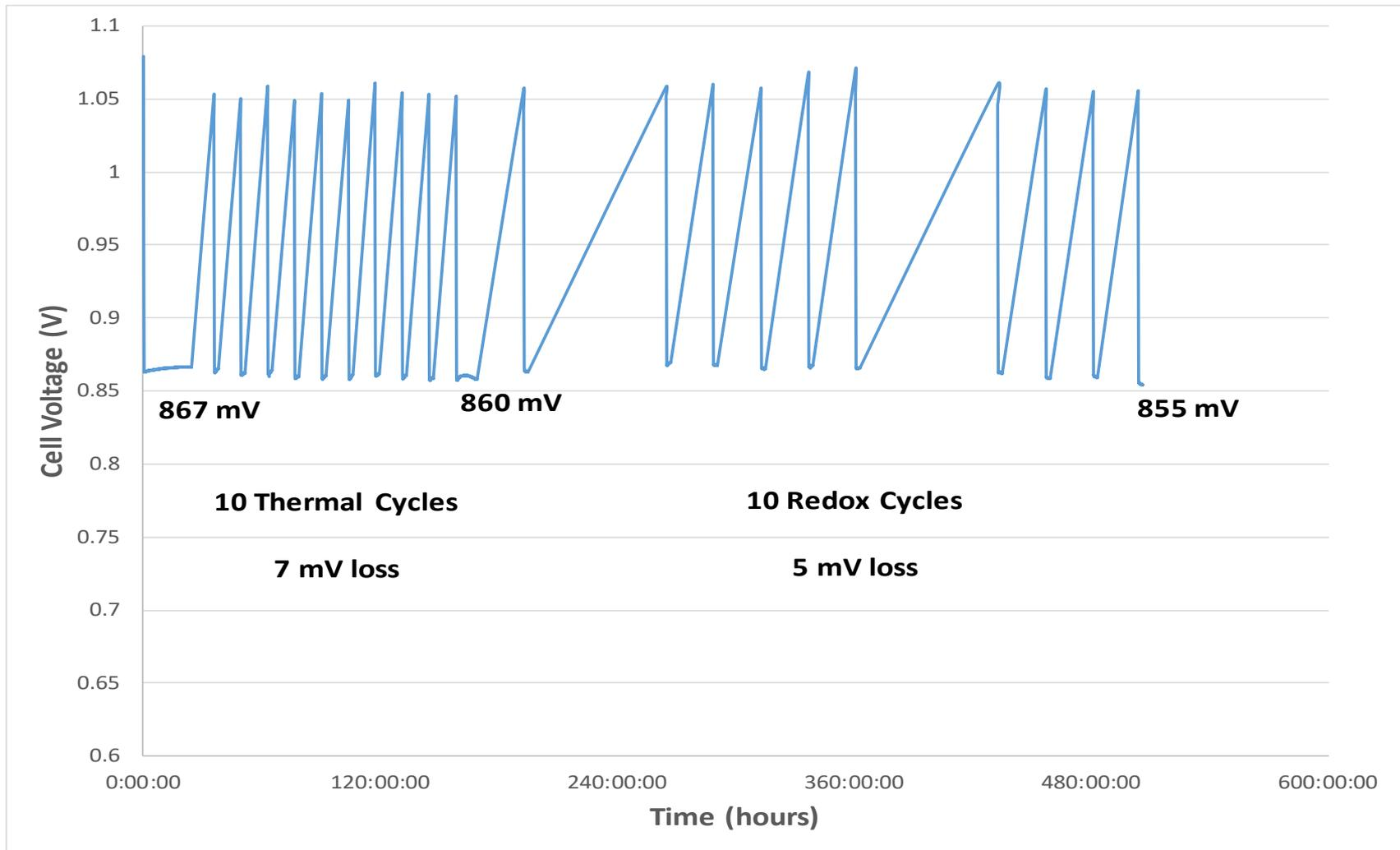
**Steady State Hold Results at 750°C over 10 Thermal and 10 Redox Shutdown Cycles With 5 Hour Hot Holds (Fuel Pipes Disconnected)**
