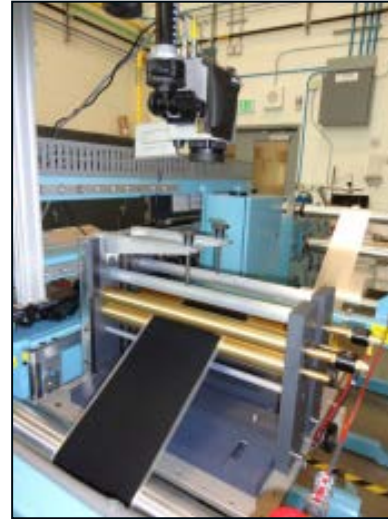
Infrared imaging of electrode and MEA defects
