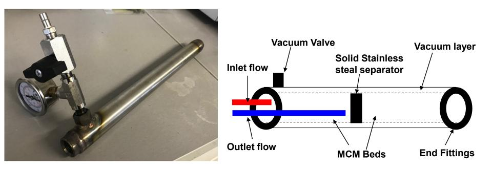
Custom vacuum jacketed MCE container design (new patent application filed!). This is a dual container that has an inner tube insulated by a vacuum layer. The magnet oscillates back and forth across the two containers. Feedthru piping is installed on each end to allow inlet flow to go through the MCE bed, and flow back out the same end.
