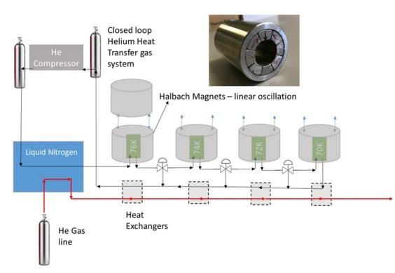
LN2 is easiest heat sink for prototype
