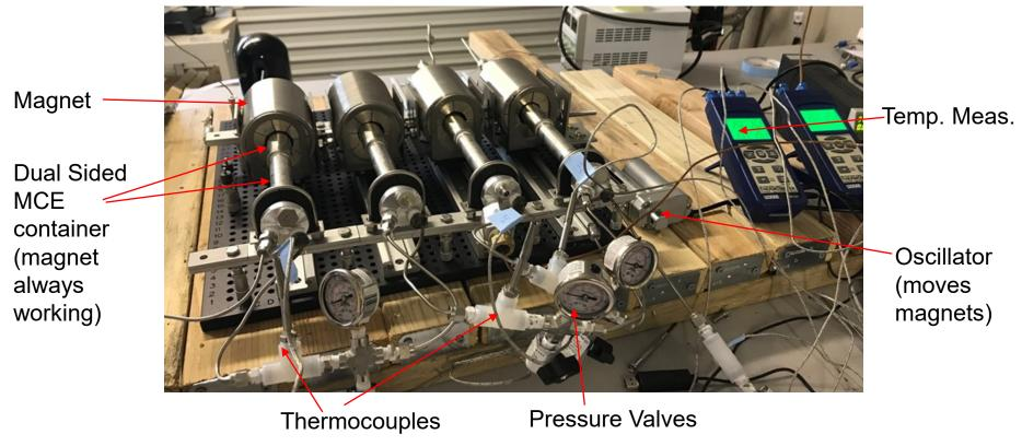
■ Initial system built and tested using room temperature MCE (Gadolinium) and mostly off the shelf parts
