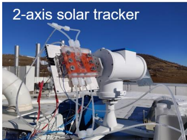
Photoreactor setup on a 2 axis solar tracker including gas collection syringe.
