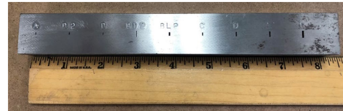
Calibration block of manufactured defects
