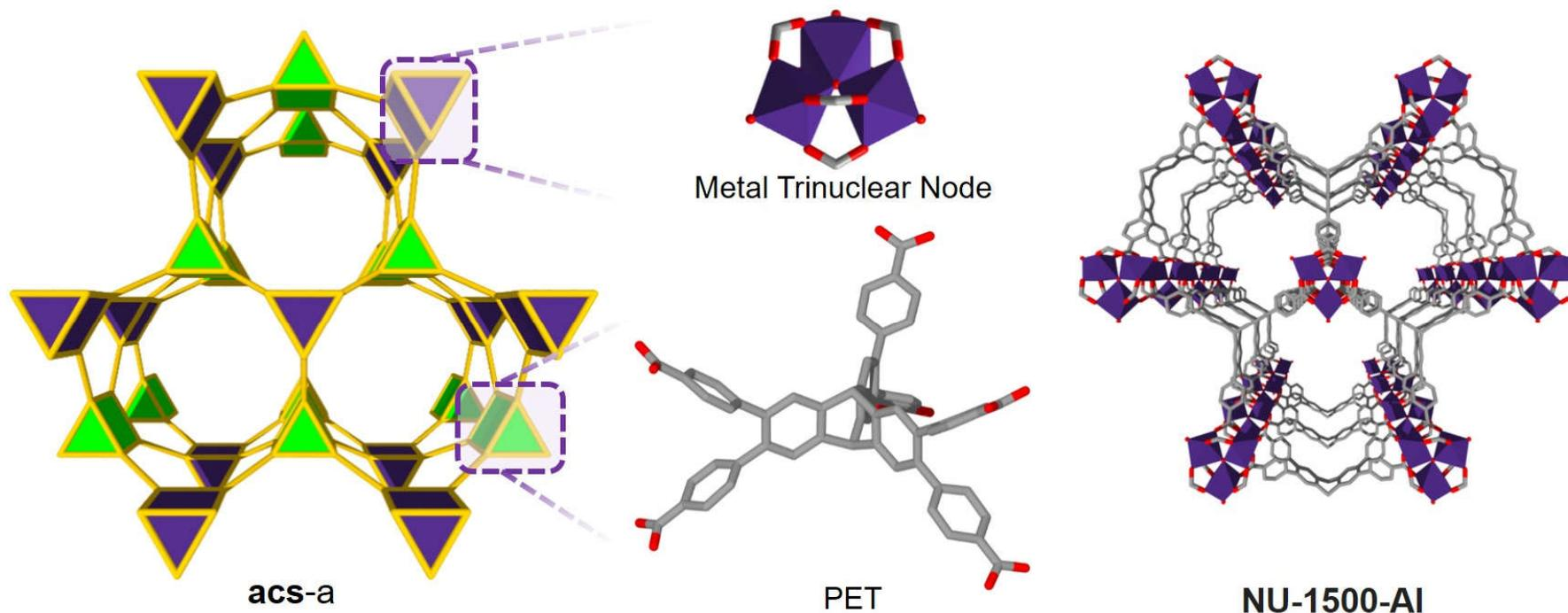
An isorecticular Al-based analogue of NU-1500-Fe was synthesized and showed high surface area.
