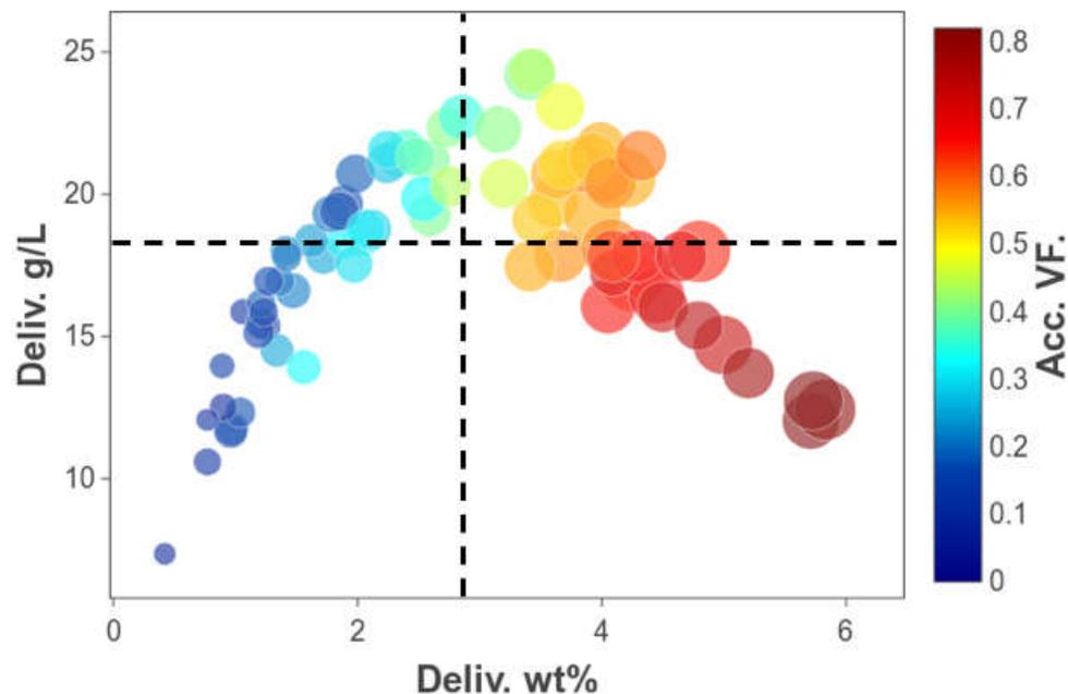
A total of 20 MOFs were able to meet both Year 1 targets (2.8 wt% and 18 g/L) simultaneously at this working condition. More are expected for the pressure-temperature swing from (233 K, 100 bar) to (296 K, 5 bar).
