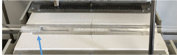
Al Foam in Furnace Tubes
