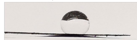
Catalyst-filled 50% PTFE Toray TGP TGP-H-030
