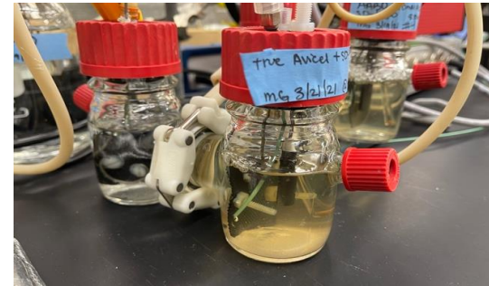
H-type microbial electrolysis cell for fermentation effluent conversion to H_2
