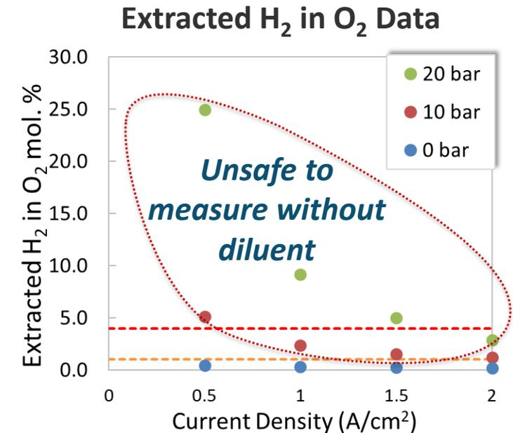
**High H<sub>2</sub> content in O<sub>2</sub> stream mitigated with inert carrier gas, enabling safe measurement of high gas crossover**
