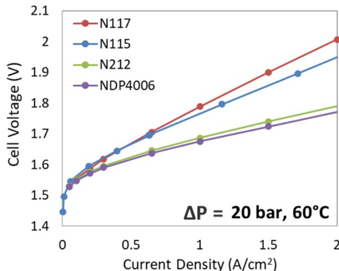
**Reinforced prototype membrane matches NR212 performance, with higher strength and reduced planar expansion**
