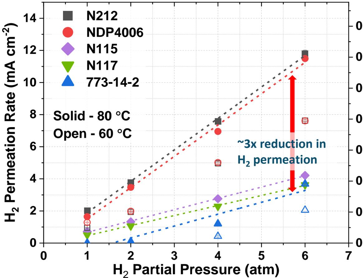
Active area: 50 cm<sup>2</sup>, Cell temperature: 80 °C, O<sub>2</sub> partial pressure: 1 atm, titanium single serpentine flow field
