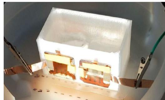
**3D-Printed PEC Reactor**
