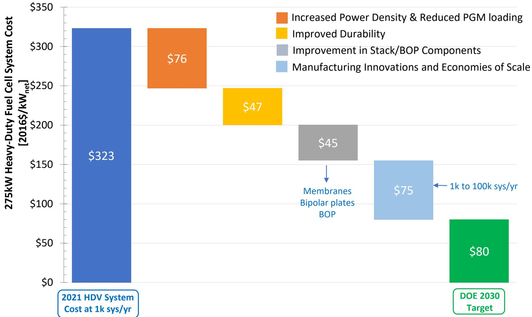
*Substantial improvements needed in power density, durability, stack and BOP components, and manufacturing.*
