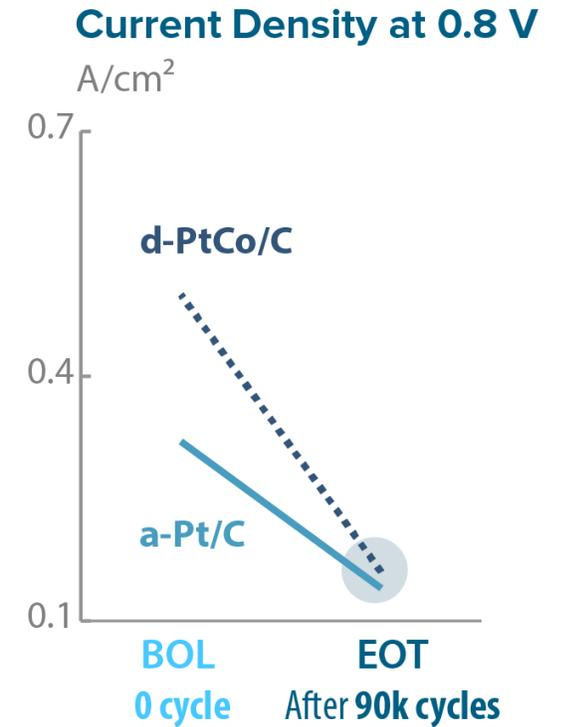
Annealed Pt/C (a-Pt/C) chosen as the baseline to meet durability and current density requirements.
