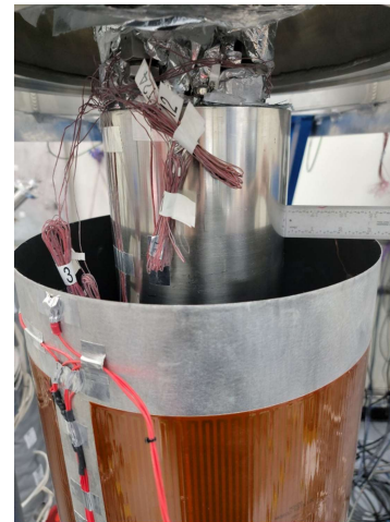
Large diameter heater sleeve ~3" insulation thickness
