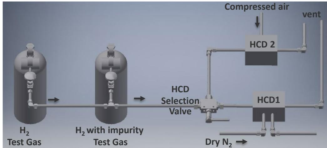
The Test Gas Generation System produces a range of contamination levels for HCD validation and calibration
