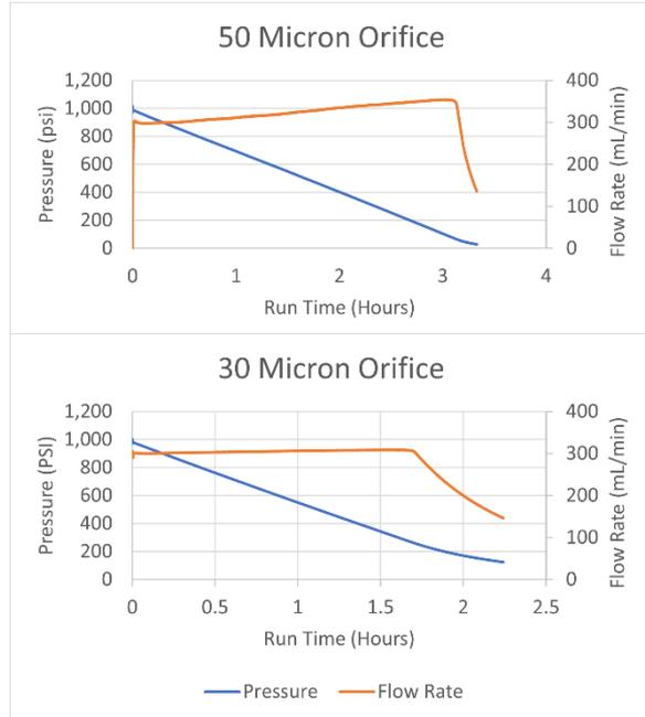
Upper: 50-micron orifice sample run
