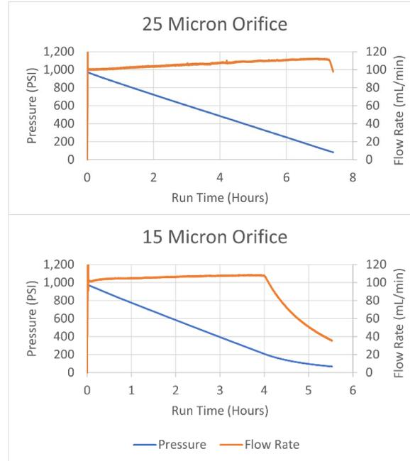
Upper: 25-micron orifice sample run
