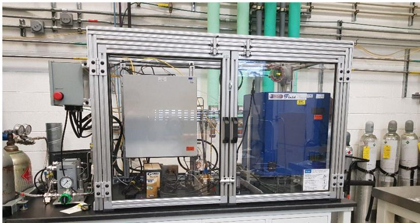
*HCD test system with an electrochemical sensor (left) and an FTIR (right) inside an enclosure providing compliance to Class 1 Division 2 operation*
