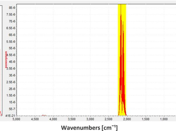
FTIR provides selective quantitation of multiple potential hydrogen contaminants
