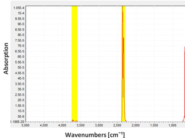
Absorption spectrum for carbon monoxide
