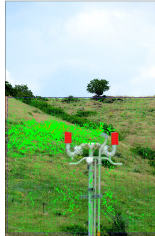
Background Oriented Schlieren Imaging of a hydrogen vent stack at NREL
